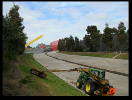
7.7m Reach arm mower with flail head and saw blade head for overhead vegetation control
