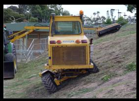
The Hustler 6400 Hillsider outfront mower has a tilting cabin to keep the centre of gravity low, it is equipped with a six foot rear discharge deck
